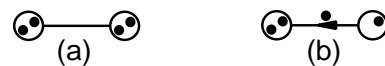
Figure 10 Example of assigning a pebble to an edge (constraint) (a) Two pebbles should be at the end vertices. (b) The constraint was added and the edge is directed.
